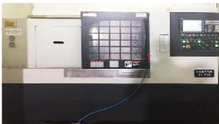
CNC TURNING CENTRE TL250: 490mm Swing Over Bed x 360mm Turning Dia With 250mm Chuck Dia
